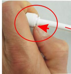
Remove the blue c-ring. Hold the elbow as shown below. Press nail toward the elbow. The same time use another hand to pull tubing out.
