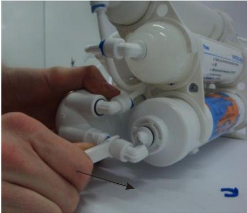
Step 2. Insert collet tool between both fittings and push it right as shown on picture. Disconnect broken part from the tubing
