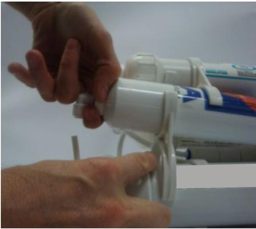
Step #4. Lift one side of the second stage filter approx. 1" up. You can hold membrane housing with another hand
