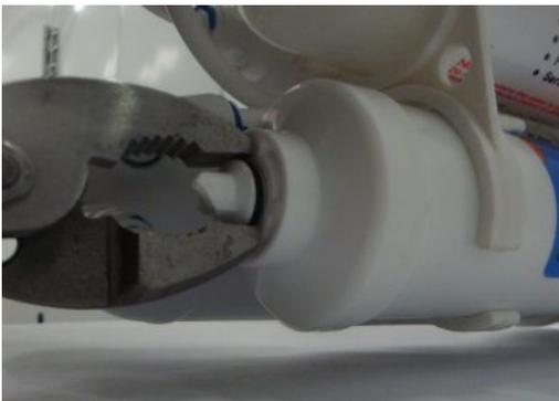
Step 3. Use pliers or scissors to remove the second part of the broken fitting
