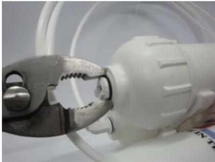
Step 3. Unscrew (counter clockwise) broken fitting using pliers. Some fitting breaks down at the base, and it is difficult to grab it with pliers. You can use scissors leg instead.
