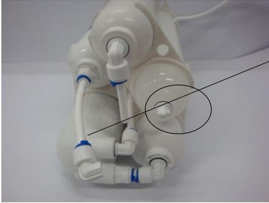
Step 1. Remove blue C-ring from the broken fitting
