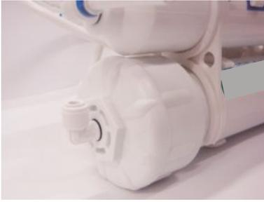
Step 5. Screw new fitting onto the head
